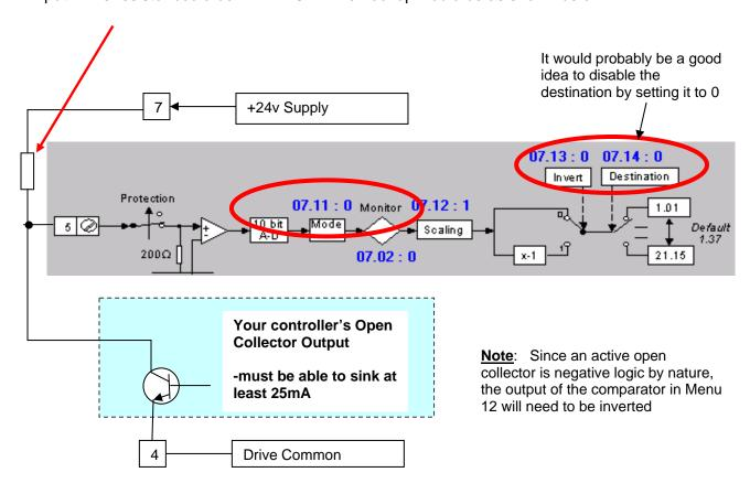
You could check to see if your input is working by observing parameter #7.02. It should be about 0.0 when your switch is open and about 100.0 when closed.
