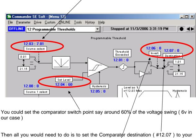
Then all you would need to do is to set the Comparator destination (#12.07) to your point of interest that you wish to control. Don't forget to depress the Red Reset button on the drive or use Reset Drive under the Tools pull down menu within SEsoft.
